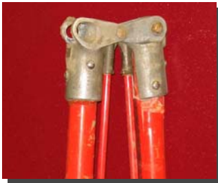
Broken Pole Stock
